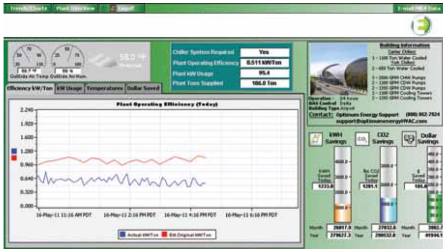
OptimumMVM shows real-time operating efficiency, daily and monthly dollars saved, and CO 2 reduction levels, and is accessible to both airport technical staff and Optimum Energy engineers.
